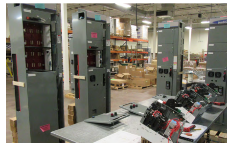
Custom-Fabricated Motor Control Centers with components being wired and pre-tested prior to final installation.
